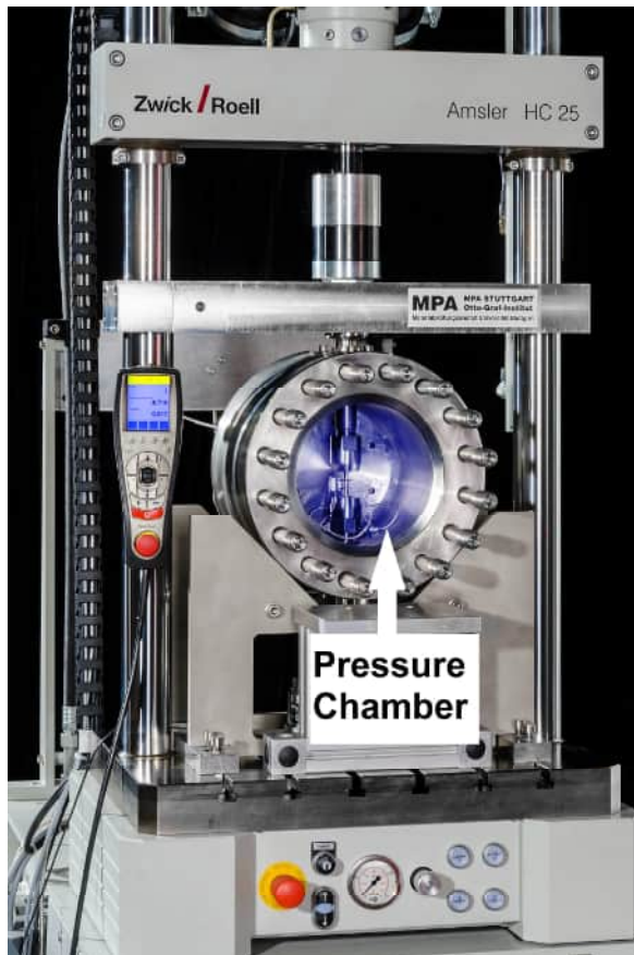
Figure 2.4: Servohydraulic testing system of MPA Stuttgart using an integrated hydrogen autoclave
