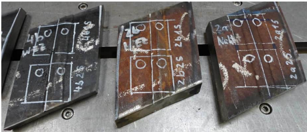
Figure 2.3: Removal of samples from a spiral welded pipe
